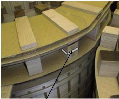
Fiber optic “F” sensor mounted in winding insulation structure directly measures factory preset and operational change in transformer short-circuit withstand capability
